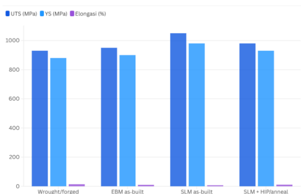
grafik 1 – Strength–Ductility Ti-6Al-4V EBM/SLM vs konvensional
