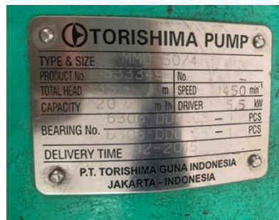
Gambar 3. Nameplate pompa Torishima
