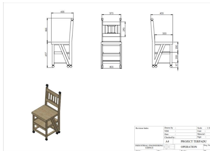
Fig. 2 2D Design of Multifunctional Folding Chair
