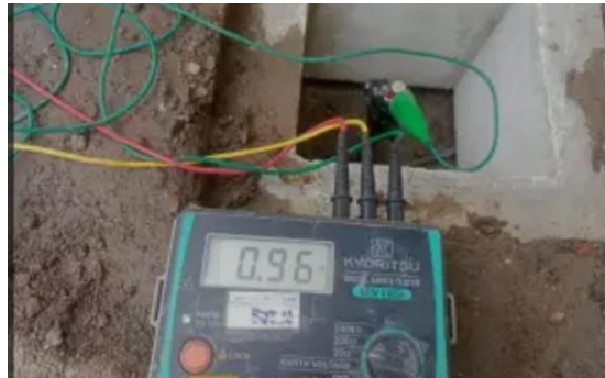
Fig. 3. The result of repairing and adding electrodes to the Server panel
