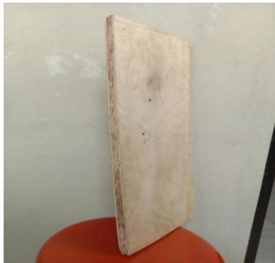
**Gambar 5. Papan Blockboard Dari Batang Kelapa Sawit**
