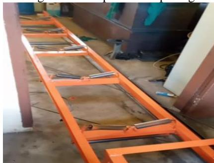
**Gambar** Rangka *Belt Conveyor*
