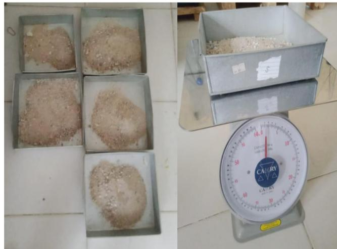
**Gambar** Proses penimbangan pasir
