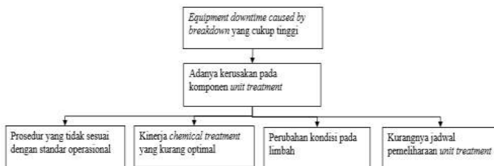
Figure 3. Root Cause Analysis on Equipment downtime caused by breakdown
