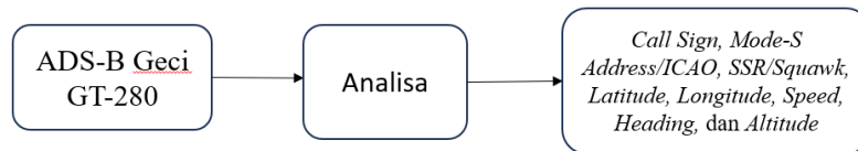
Gambar III. 5 Ilustrasi Pengambilan Data ADS-B Geci GT-280
