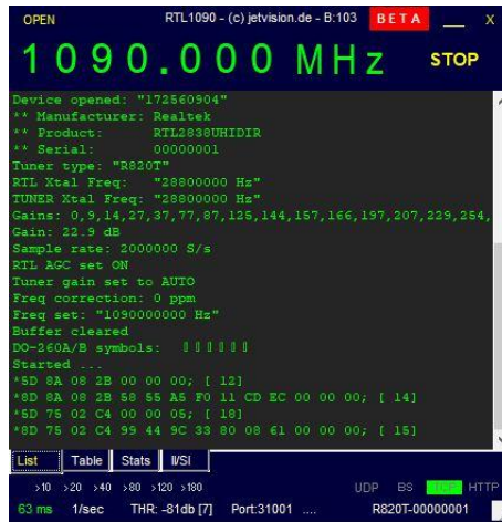
Gambar IV. 1 Tampilan RTL-SDR V3 Menerima Data Asterix
