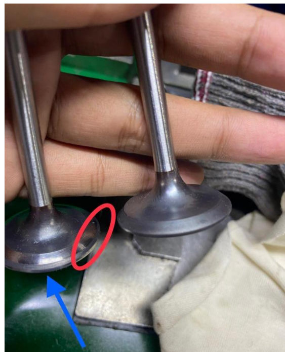
Gambar 2. Defect Face Uncut di Engine Valve Sumber : PT. XYZ, 2022
