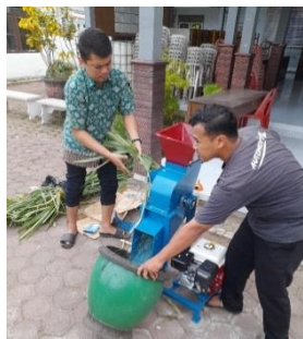
Gambar 3. Uji Coba Teknologi Portable Chopping Grass Machine
