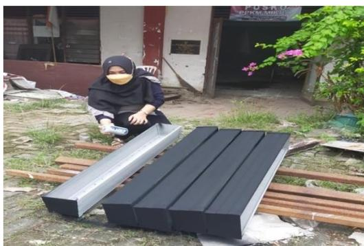
Gambar 4 Proses Pengecatan Talang PVC
