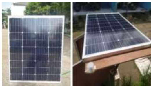
Gambar 3. Perancangan Panel Surya 100 Wp Berjenis Monocrystalline
