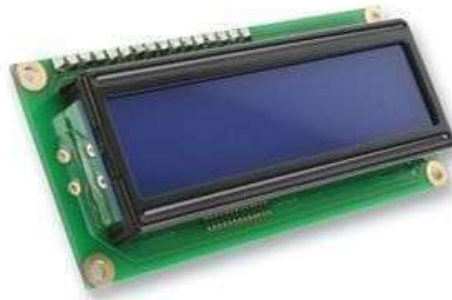
Gambar 11. Liquid Cristal Display (LCD)
