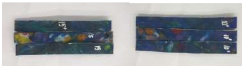
Gambar 7 Specimen ASTM D 3039
