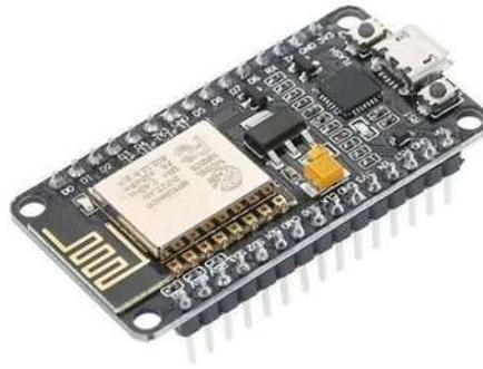
**Gambar 2.1 NodeMCU ESP8266**
