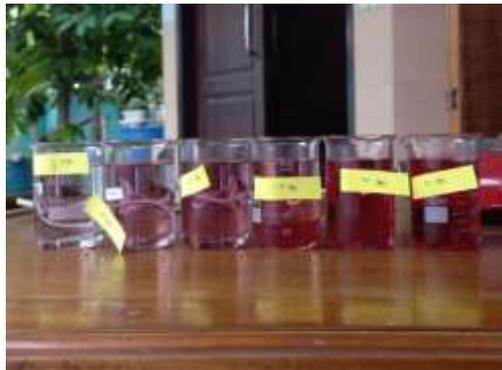
Figure 2. Synthesis of nanogold with various concentrations of 5,10,15,20,25 and 30 ppm
