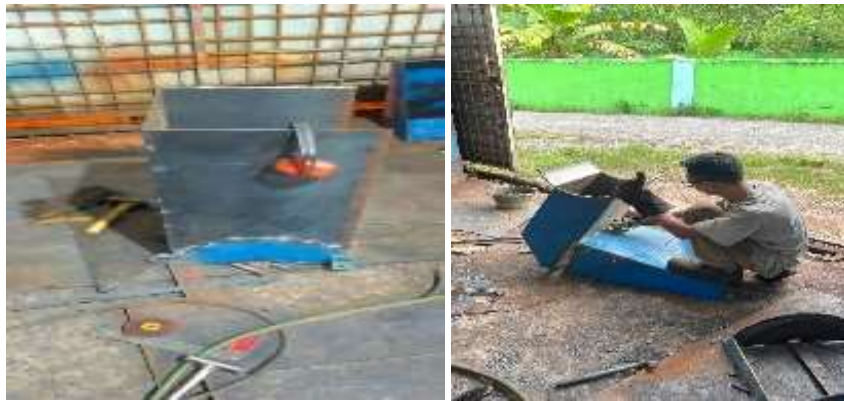
Gambar 7. Fabrikasi Mesin Pencacah Plastik di workshop CV Star Umroh Engineering.
